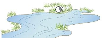
2) Encapsulating an outfall within watercourse bank using geotextiles
