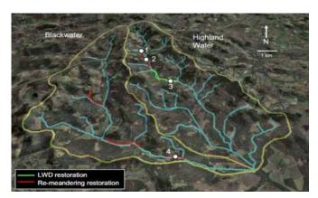
LIFE-3 project catchments showing the locations of channel/ floodplain restoration and the main monitoring reaches. 1 = Semi-natural Control,
