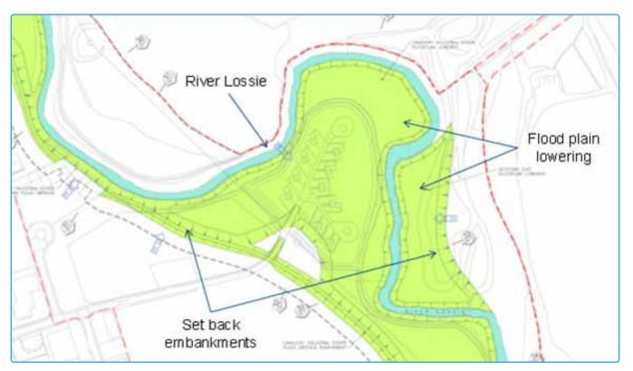
Example design of the Elgin Flood Alleviation Scheme. This section indicates the floodplain lowering and set back embankments used around the Moycroft and Chanonry section of the River Lossie. The full scheme involved modification to 1.5km of the River Lossie, Tyock Burn and Linkwood Burn.
